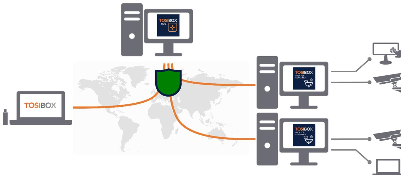
Figure 3: Connectivity from Tosibox Key Client to devices behind Tosibox Lock for Container via Tosibox HUB
