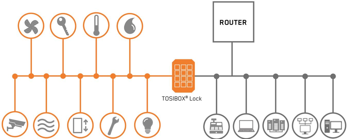
Systems connected to TOSIBOX® Lock router device that subcontractors can connect to with TOSIBOX® Key.
