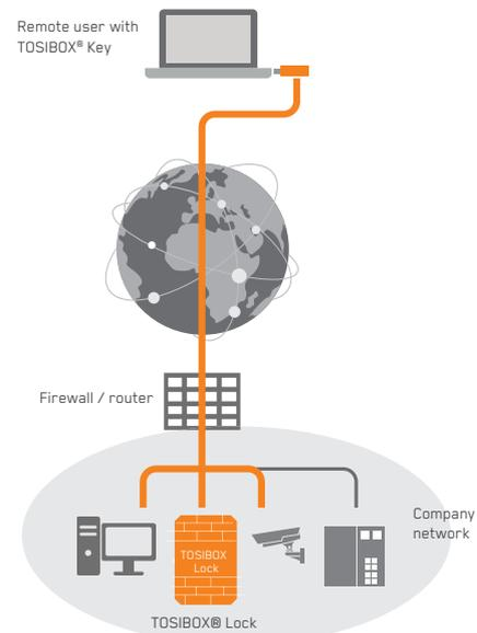
In both cases the Lock will use the company network to get access to the Internet. This usually doesn't require any special configuration or firewall changes. The rule of thumb is that if you can access the Internet freely from your network, remote access with TOSIBOX<sup>®</sup> Lock will also work. Thanks to the patented connection method, TOSIBOX<sup>®</sup> is firewall and NAT friendly and typically no ports need to be opened on the company firewall for the VPN connection to work.
