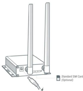
1. Connect the operating voltage of 9-35 V DC to the device and wait for few seconds.
